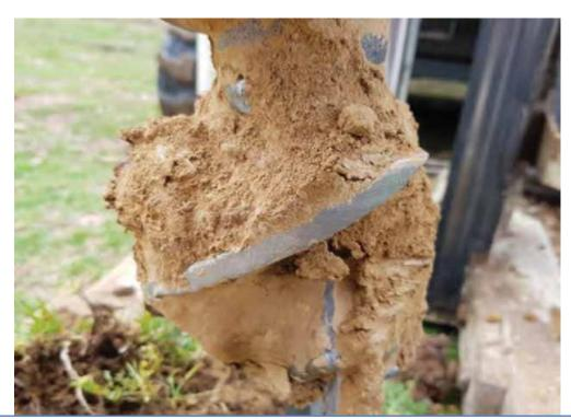
Plate 12 – Natural soils observed at depth of 1.5 mBGL in bore hole TP15.
