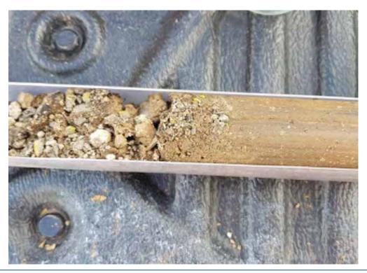
Plate 7 – Soil materials observed at depth of 0.15 mBGL in bore hole TP3.
