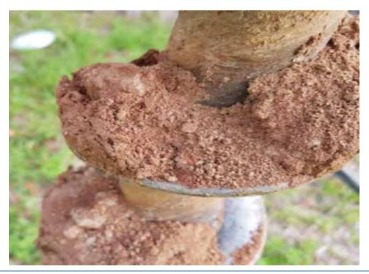
Plate 9 – Soil materials observed at depth of 0.5 mBGL in bore hole TP17.
