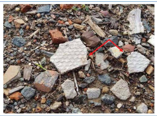
Plate 6 – Asbestos fibre cement debris observed at the north-eastern side of the Site.
