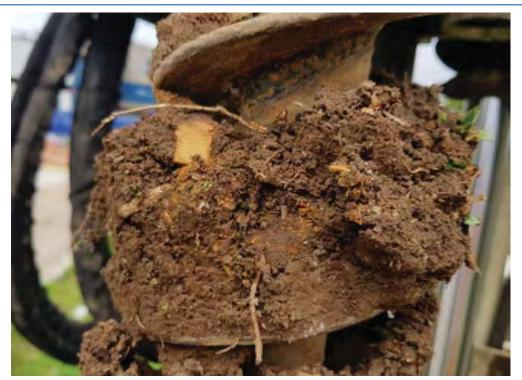
Plate 8 – Soil materials observed at depth of 0.15 mBGL in bore hole TP9.
