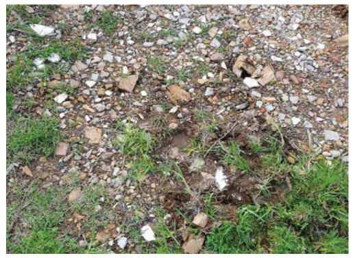
Plate 13 – Crushed concrete and debris intermixed with fill materials at eastern side of the Site. Date: 15/10/2018
